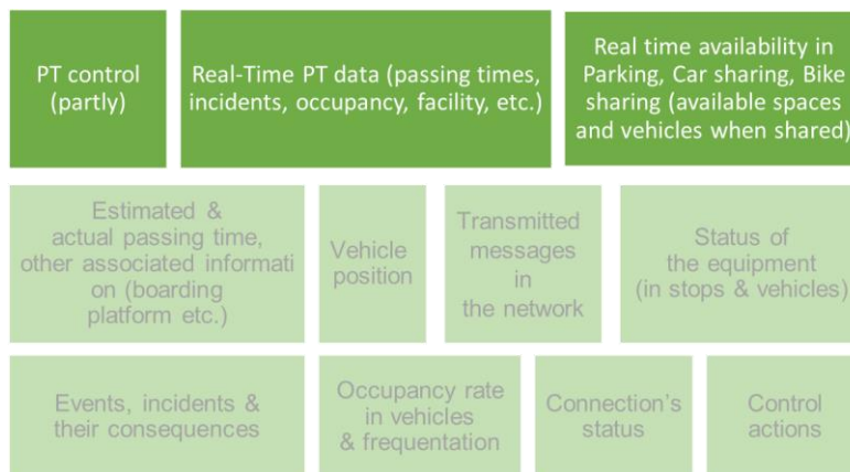
Figure 3.4 Functional scope of SIRI (data categories and subcategories - in light green). Source DATA4PT
